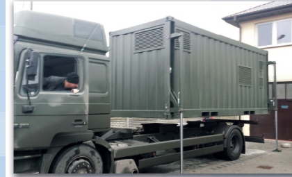
Container with self-lifting system
